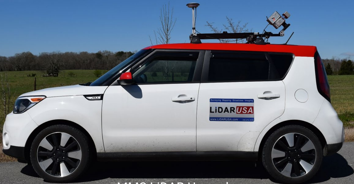
MMS LiDAR Upgrade
